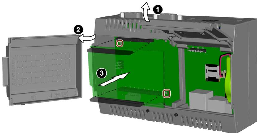
2. Open the cover on the left by slightly raising the cover and lifting it to the left.
